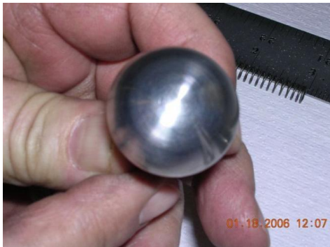
Photo 3.0 (Dart after 800 bbl liquid flow test)
