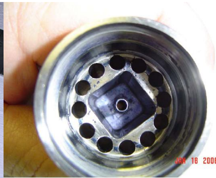
Photo 4.0 (Nose ID after 800 bbl liquid flow test)
