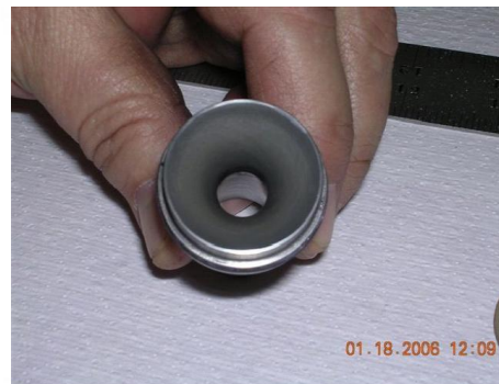
Photo 7.0 (Venturi Orifice after 800 bbl liquid flow test)
